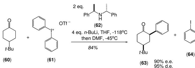
**Scheme 2.3:** Asymmetric  $\alpha$ -arylation of 4-(*tert*-butyl)cyclohexanone (**60**) with diphenyl iodonium salt **61** employing chiral base **62**
