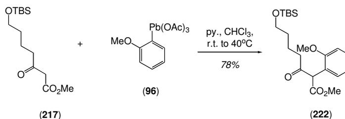
**Scheme 3.9:**  $\alpha$ -Arylation of  $\beta$ -ketoester **217** with *o*-methoxyphenyllead triacetate (**96**) to synthesise  $\alpha$ -arylated  $\beta$ -ketoester **222**
