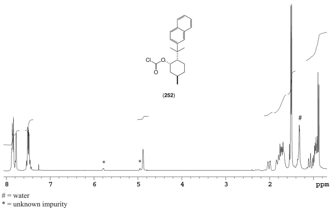
**Figure 4.2:** 300 MHz  $^1\text{H}$  NMR spectrum of chloroformate **252** recorded in  $\text{CDCl}_3$  at  $18^\circ\text{C}$
