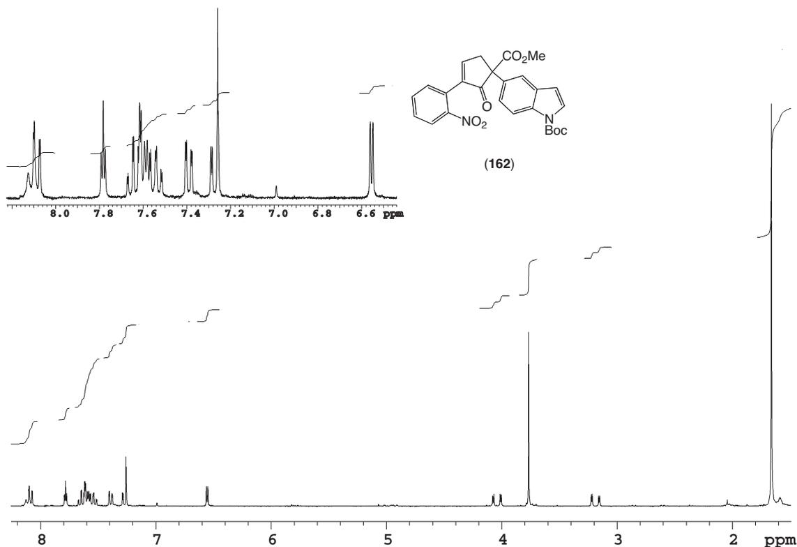
**Figure 2.10:** 300 MHz  $^1\text{H}$  NMR spectrum of nitro-arene **162** recorded in  $\text{CDCl}_3$  at  $18^\circ\text{C}$
