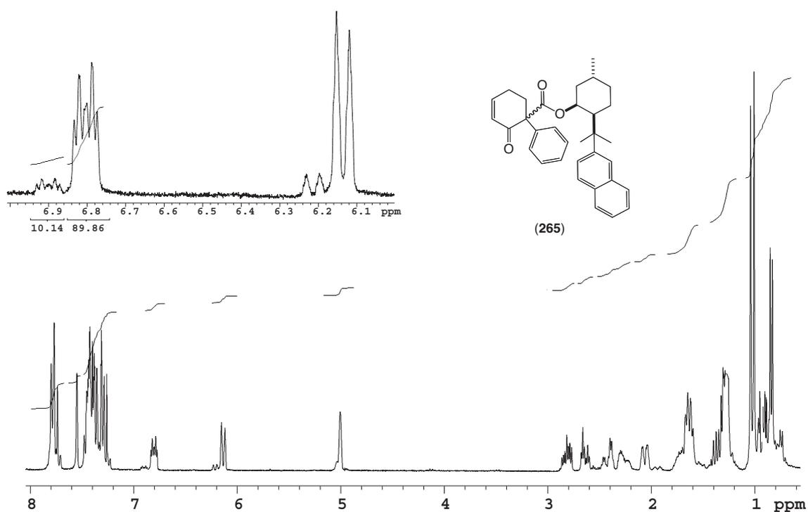
**Figure 4.6:**  $300\text{ MHz } ^1\text{H}$  NMR spectrum of  $\alpha$ -arylated enone **265** recorded in  $\text{CDCl}_3$  at  $18^\circ\text{C}$  (doubling of signals due to presence of diastereoisomers)
