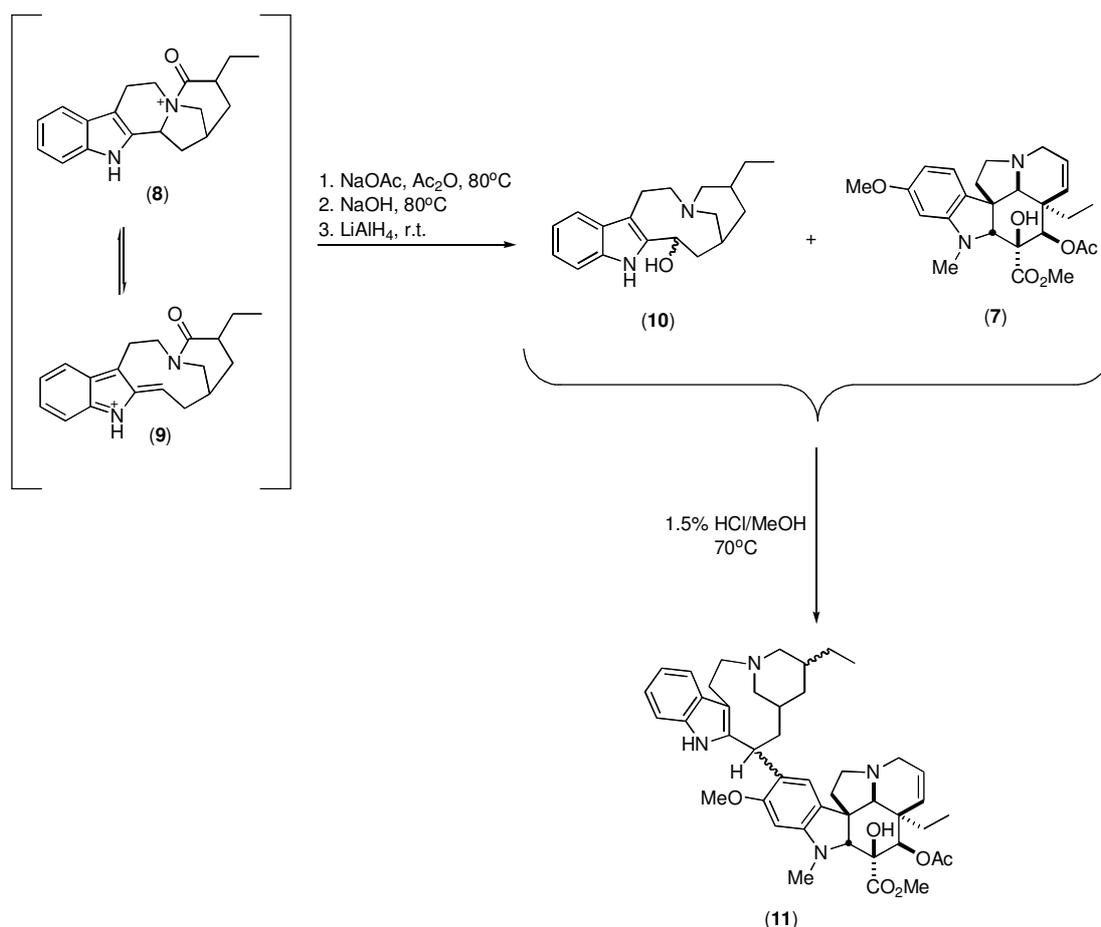
**Scheme 1.2:** Key elements associated with the hydroxyindole approach to the binary indole-indoline alkaloids
