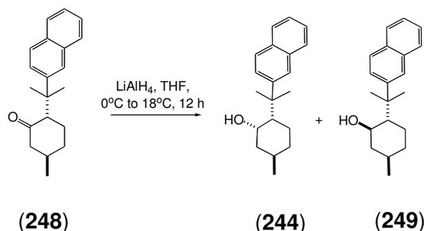
Following a procedure developed by Yang *et al.*<sup>21</sup> a magnetically stirred and cooled (ice/water bath) solution of cyclohexanone **248** (800 mg, 2.86 mmol) in THF (5 mL) under a nitrogen atmosphere was treated with LiAlH<sub>4</sub> (5.74 mL of a 1 M solution in THF, 5.74 mmol). The resulting mixture was warmed to 18°C, stirred at this temperature for 12 h, then quenched with ammonium chloride (1 x 5 mL of a saturated
