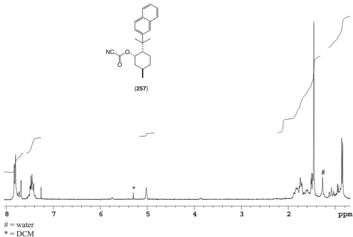
**Figure 4.4:** 300 MHz  $^1\text{H}$  NMR spectrum of cyanoformate **257** recorded in  $\text{CDCl}_3$  at  $18^\circ\text{C}$
