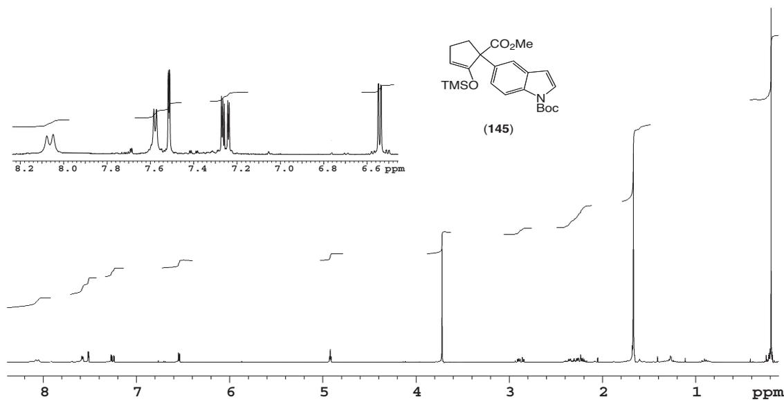
**Figure 2.4:** 300 MHz  $^1\text{H}$  NMR spectrum of trimethylsilylenol ether **145** recorded in  $\text{CDCl}_3$  at 18 °C
