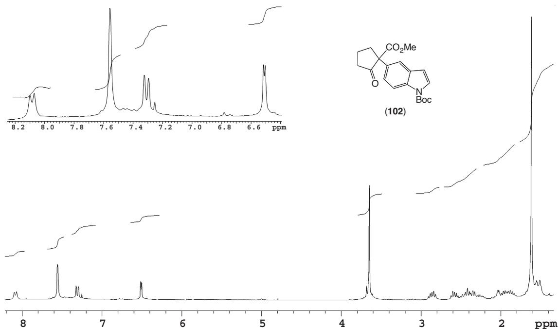
**Figure 2.2:** 300 MHz  $^1\text{H}$  NMR spectrum of  $\alpha$ -arylated  $\beta$ -ketoester **102** recorded in  $\text{CDCl}_3$  at 18  $^\circ\text{C}$  (line broadening attributed to the presence of carbamate rotomers)
