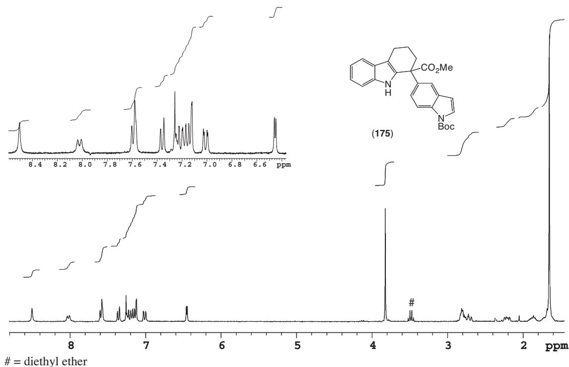
**Figure 2.12:** 300 MHz  $^1\text{H}$  NMR spectrum of indole **175** recorded in  $\text{CDCl}_3$  at 18 °C
