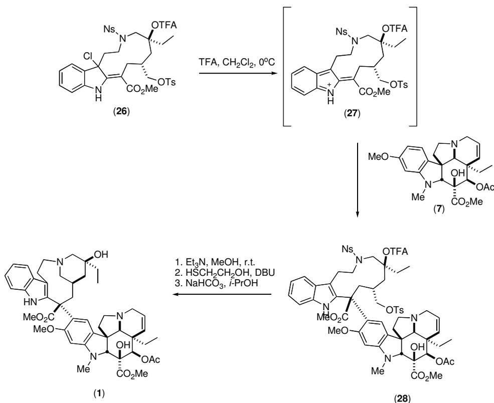
**Scheme 1.7:** The late stages of Fukuyama's stereocontrolled total synthesis of (+)-vinblastine (**1**) involving chloroindolenine **26** as a precursor to the coupling species **27**
