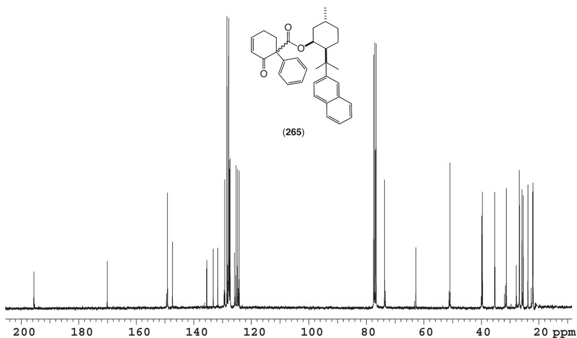
**Figure 4.7:**  $75\text{ MHz } ^{13}\text{C}$  NMR spectrum of  $\alpha$ -arylated enone **265** recorded in  $\text{CDCl}_3$  at  $18^\circ\text{C}$  (doubling of signals due to presence of diastereoisomers)
