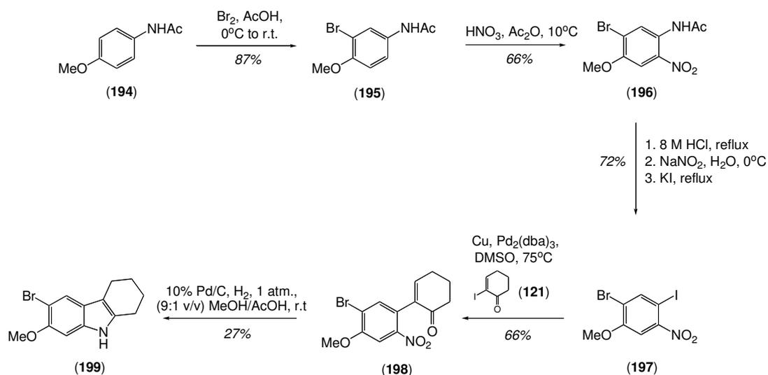
**Scheme 3.1:** Pd[0]-catalysed Ullmann cross-coupling approach to tetrahydrocarbazole **199**
