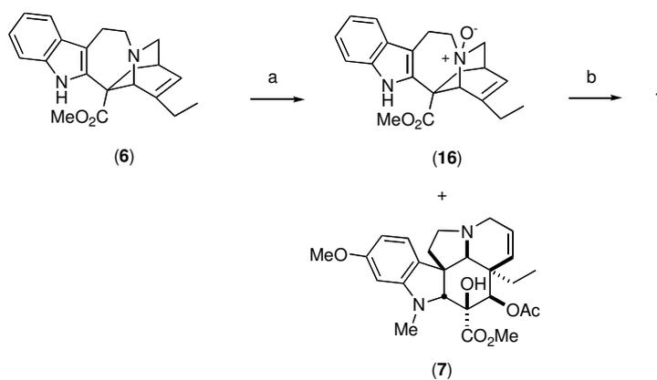
*Reagents and conditions:* (a) *m*CPBA, CH<sub>2</sub>Cl<sub>2</sub>, -30°C (b) i. TFAA, CH<sub>2</sub>Cl<sub>2</sub>, -60°C; ii. β-NADH, MeOH, r.t.; iii. FeCl<sub>3</sub>, O<sub>2</sub>, MeOH, 0°C; iv. NaBH<sub>4</sub>, MeOH, r.t.
