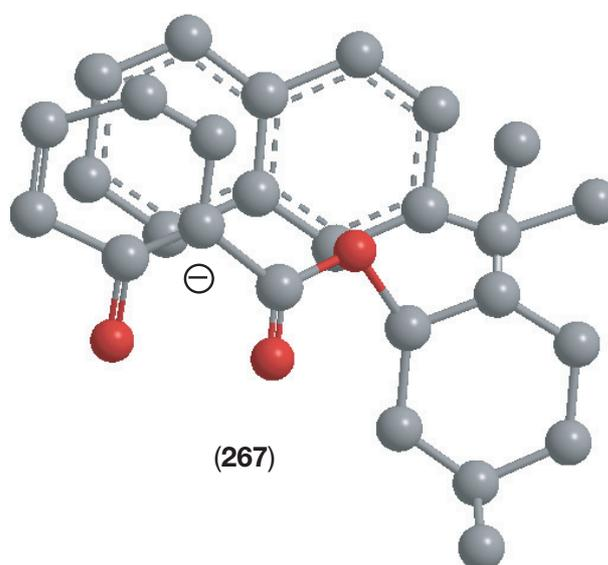
*Figure 4.8: Proposed conformation of enolate **267** with a  $\pi$ -stacking interaction shielding the lower face*
