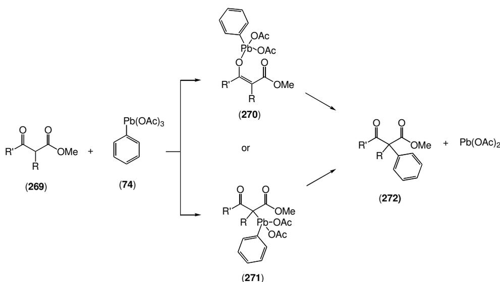
**Scheme 4.6:** Alternative intermediates in the  $\alpha$ -arylation of  $\beta$ -ketoesters **269** with phenyllead triacetate (**74**)
