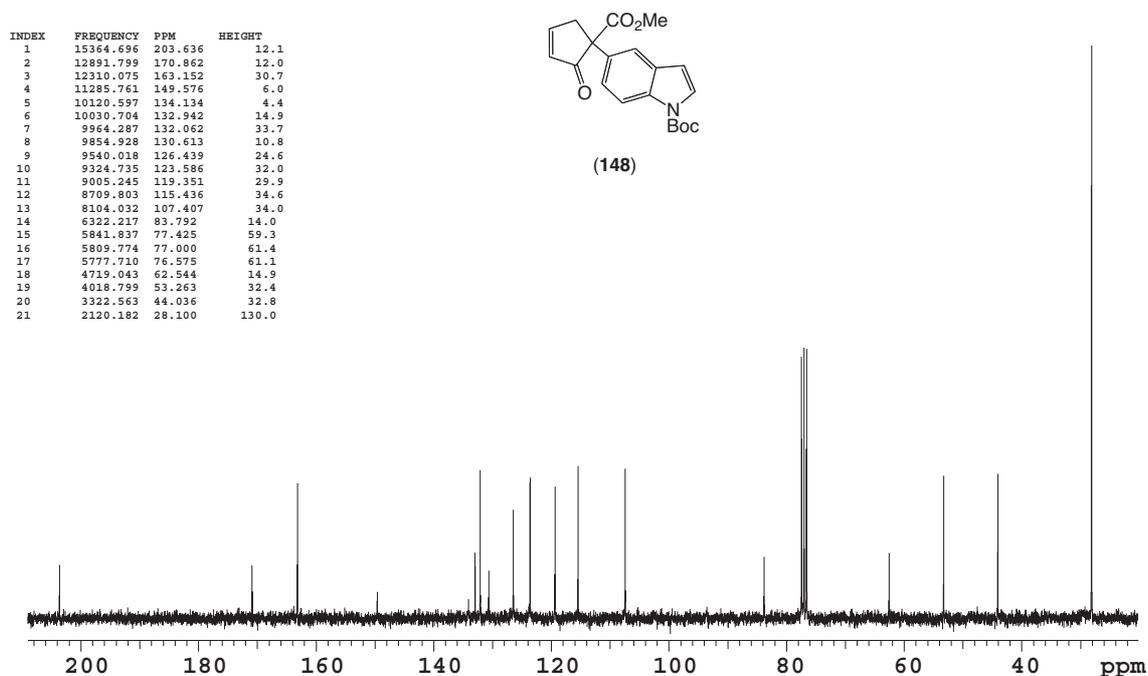
**Figure 2.7:** 75 MHz  $^{13}\text{C}$  NMR spectrum of enone **148** recorded in  $\text{CDCl}_3$  at 18 °C
