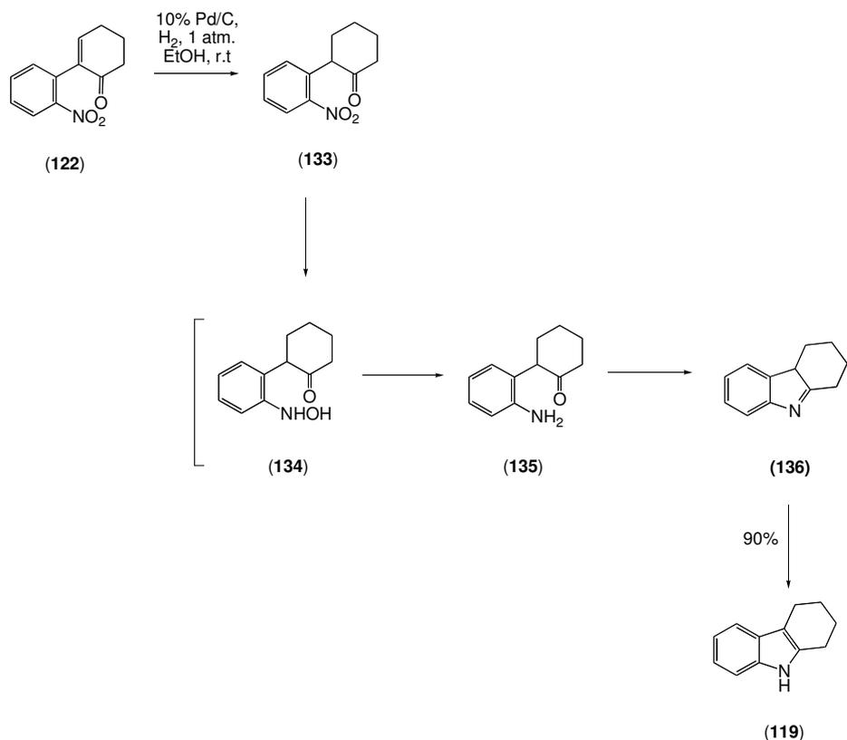
**Scheme 2.13:** Proposed mechanism associated with the reductive cyclisation of nitro-arene **122** to tetrahydrocarbazole **119**
