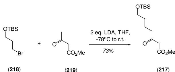
**Scheme 3.8:** Synthesis of  $\beta$ -ketoester **217**
