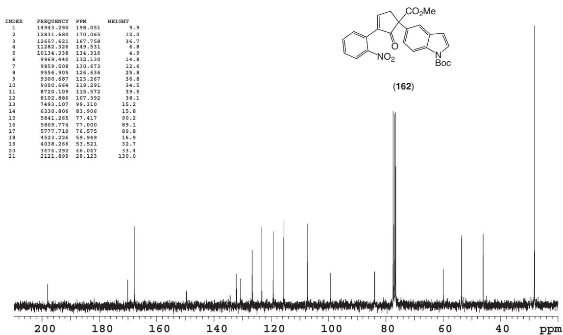
**Figure 2.11:** 75 MHz  $^{13}\text{C}$  NMR spectrum of nitro-arene **162** recorded in  $\text{CDCl}_3$  at  $18^\circ\text{C}$
