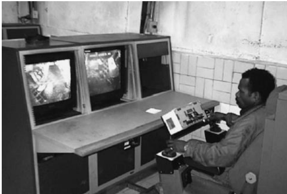
Figure 1.4: Mining telerobotics user interface from [6]
