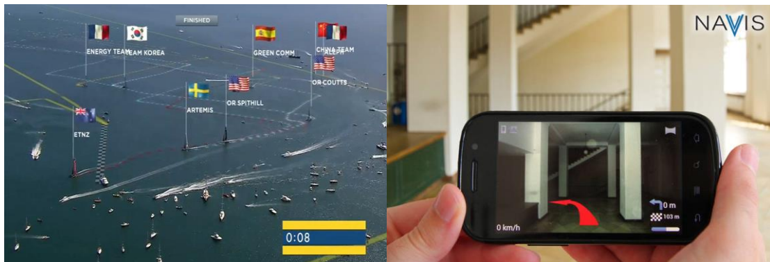
Figure 2.20: Examples of AR interfaces. (Left) Embedded country flags and the names of sailors are displayed on the screen for the America's Cup race tracking display [84], and (Right) An arrow object as additional navigation interface [85]
