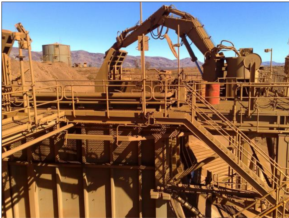
Figure 1.2: Rockbreaker robot arm from [5]
