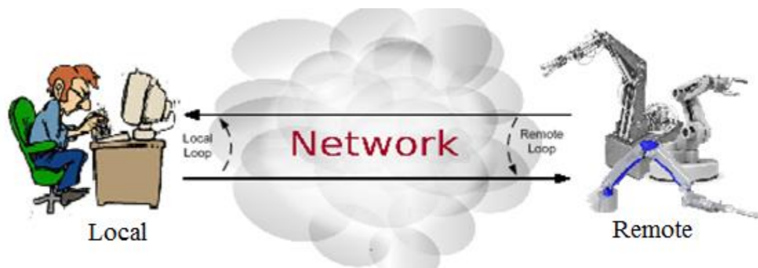
Figure 1.1: General telerobotics architecture. In the local area, the operator generates commands, performs manipulation and receives feedback from the system interface; while the remote machine performs the command, sends feedback and has some level of autonomy.
