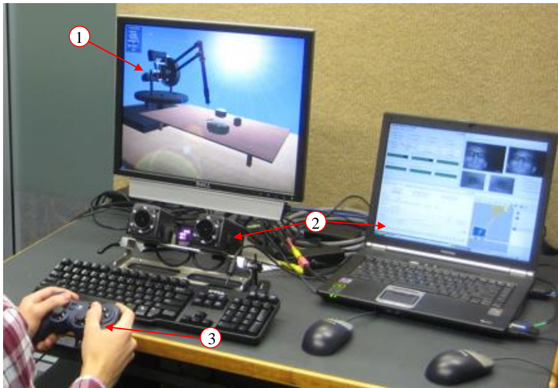
Figure 4.10: User setting: (1) Unit PC with situated virtual application running on it, (2) FaceLAB V.4.5 eye tracker software and sensors, (3) Logitech Dual Action gamepad
