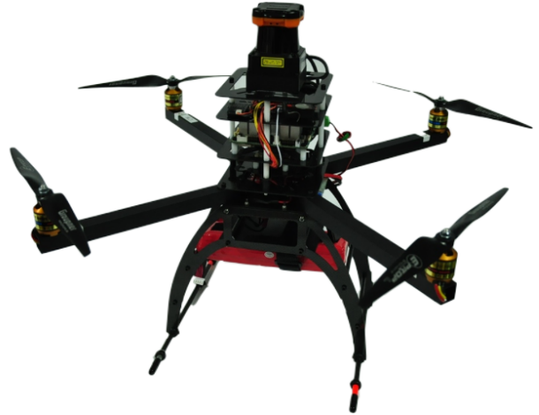
Fig. 1. A quadrotor, the multirotor vehicle considered in this paper. We propose a new motor controller that uses aerodynamic power as its desired output.
