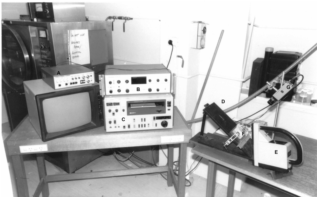
Figure 5.2: Complete setup of micromodelling experiments showing A: timer, B: video enhancer, C: video recorder, D: inclined platform, E: UV light source, F: micromodel and G: CCD camera.
