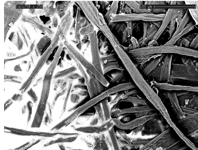
Figure 7.28: Higher magnification image of a 7.5% talc filled paper showing more detail of pore filling.
