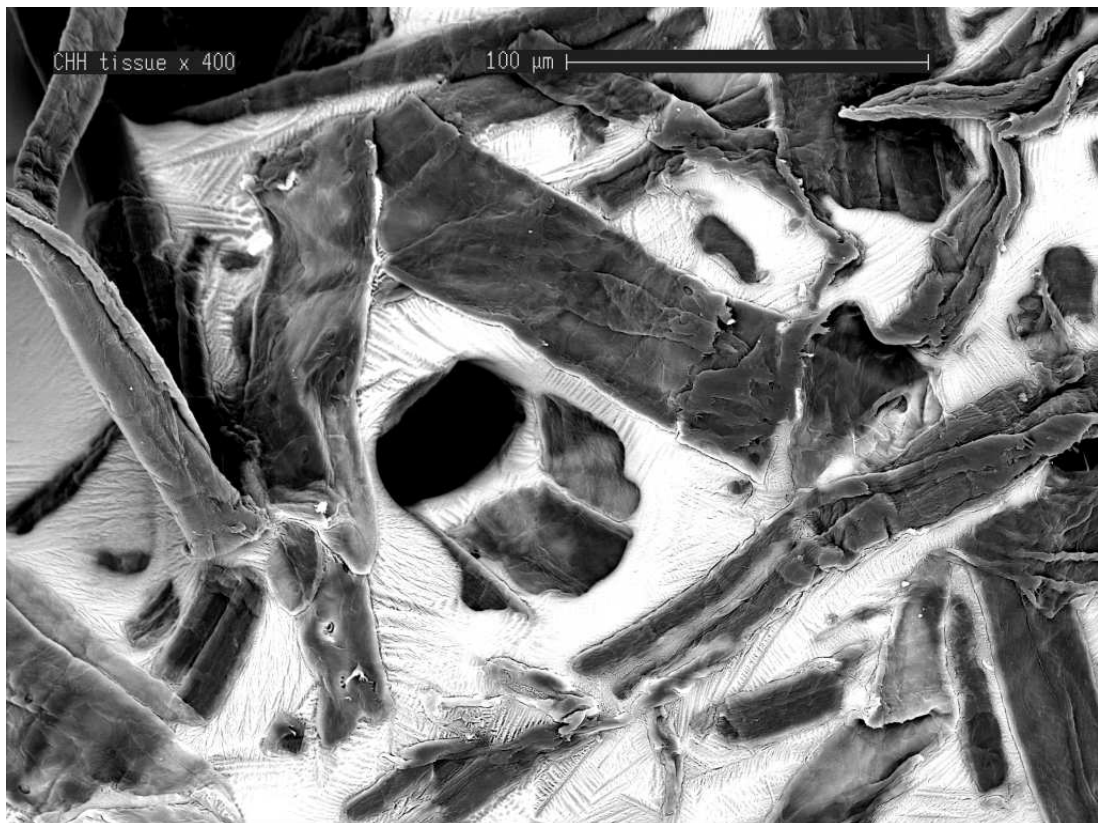
High magnification cryo-SEM image of film thickening around a large pore in tissue paper.
