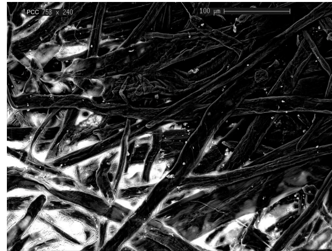
Figure 7.24: Higher magnification image of a 7.5% PCC filled paper showing infilling of pores.
