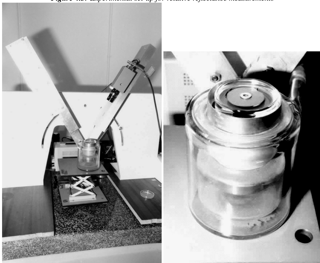
Figure 4.3: Experimental set-up for relative reflectance measurements
