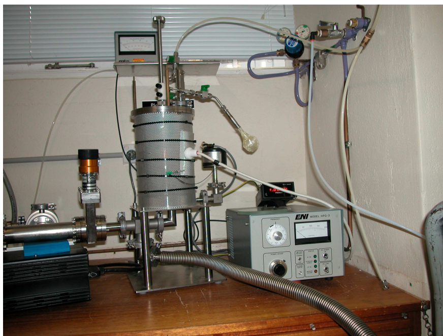
Figure 7.3: Plasma reactor setup including chamber and RF generator
