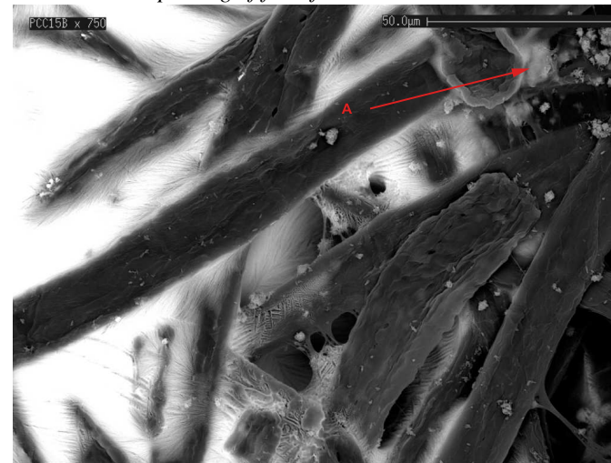
Figure 7.32: Higher magnification image of a 15% PCC filled paper showing film flow at edge of wetting area. Arrow A shows particles of PCC being readily wet and arrow B shows particles in a fibre overlap channel where pinning of fluid flow is evident.
