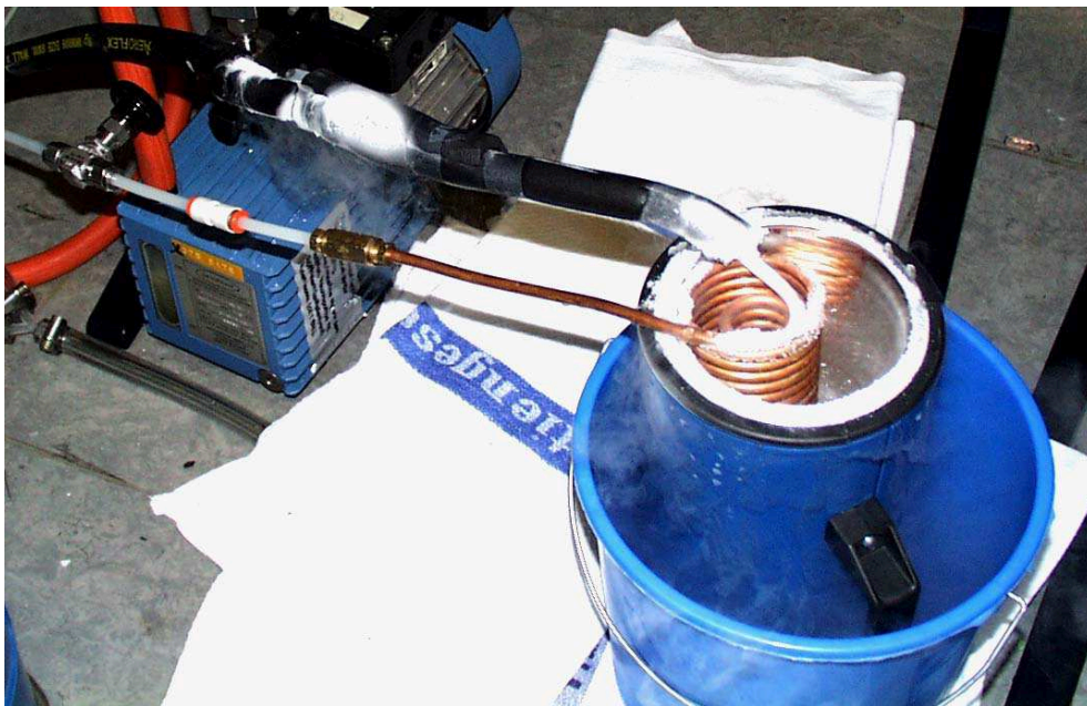
Figure C.1: Copper cooling coil placed in dewar of liquid nitrogen showing needle valve on the supply side of the nitrogen gas and the vacuum pump used for generating nitrogen slush
