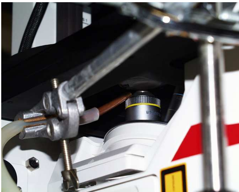
Figure 6.4: Nitrogen gas nozzle used to remove condensation from bottom window of cryo-cell
