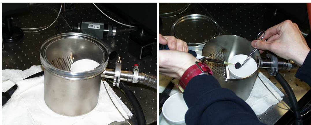
Figure 6.3: Vacuum chamber for preparation of ( SLN_2 ) and placement of droplet onto paper sample immediately prior to freezing in the chamber. This technique was exactly the same as that used for cryo-SEM except with the purpose built Oxford cryo chamber.
