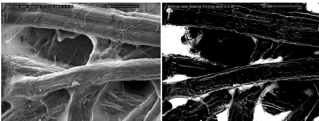
Figure 6.1: An example of an SEM image of fluid penetration into kraft paper in (a) secondary electron mode and (b) backscattered mode.
