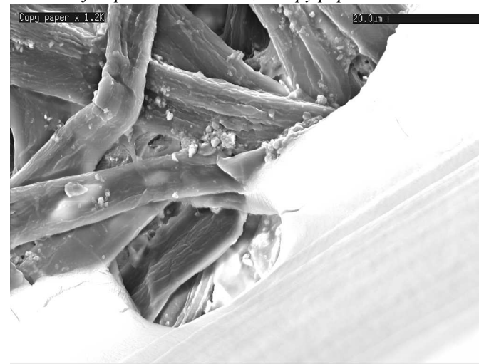
Figure 6.27: SEM secondary electron image of fluid droplet frozen 2 seconds after placement onto sized copy paper.
