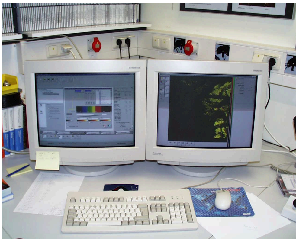
Figure 6.6: Computer station controlling two-photon microscope showing image acquisition on right screen and microscope and laser configurations on the left screen.
