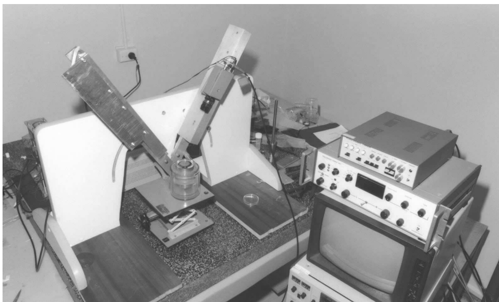
Figure 4.3: Experimental set-up for relative reflectance measurements
