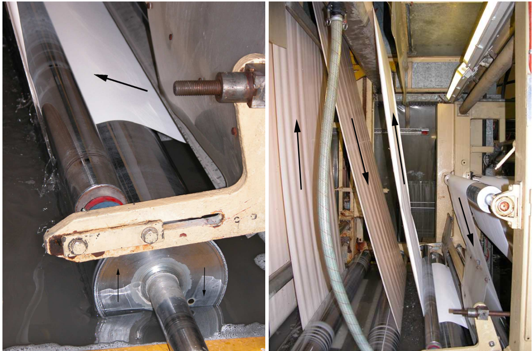
Figure 1.2: Images of pre-wetting roller, closeup on the left and showing the positions of the sky rollers on the right. Note that only the bottom third of the pre-wetting roller is in the resin bath. The roller rotates against the travel of the paper enabling a film of resin on the roller to come into contact with the paper. Arrows denote the direction of movement of the paper and the prewetting roller.
