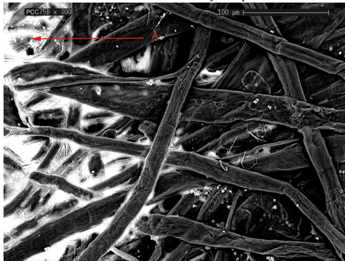
Figure 7.23: Low magnification image of wetting of paper filled with 7.5% PCC. Arrows marked A show unfilled pores.
