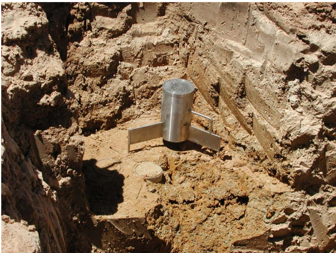
Plate 6.1 The bulk density corer used to obtain bulk density cores
