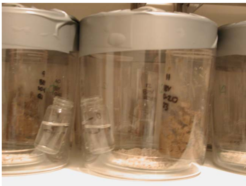
Plate 3.2 Experimental set-up used for analysis of soil respiration; incubation chamber with soil sample, vial of water and soda lime trap
