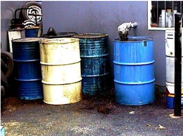
Figure 5.5a. Chemical storage with poor environmental management. Inherent environmental risk is equal to residual environmental risk.
