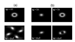
FIG. 5. Suppression of the vortex filamentation due to modulational instability in the presence of a copropagating fundamentalmode beam (see discussion in the text). Numerical results are obtained for s = 0.65 and  $\lambda = 0.5$ : (a) z = 35, (b) z = 90.
