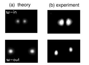
FIG. 4. (a) Results of numerical simulations showing strong repulsion of the input dipole-mode lobes without the second component. (b) Experimental results showing the strong repulsion the two out-of-phase solitons formed by the dipole lobes without the copropagating Gaussian beam [theoretical and experimental parameters as in Figs. 3(a) and 3(b)].
