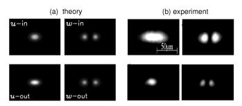
FIG. 3. (a) Results of numerical simulations showing the generation of a stable dipole-mode soliton (s = 0.65,  $\lambda = 0.5$ , z = 35). (b) Experimental results showing formation of a dipole-mode soliton (bottom) from the two outof-phase beams (top, right) and copropagating Gaussian beam (top, left). Experimental parameters are V = 2 kV, z = 15 mm, and the initial powers of the *u* and *w* components  $P_u = P_w = 0.6 \mu \text{W}$ .
